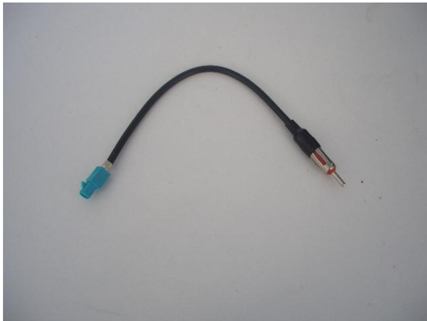
The antenna adapter for later cars
